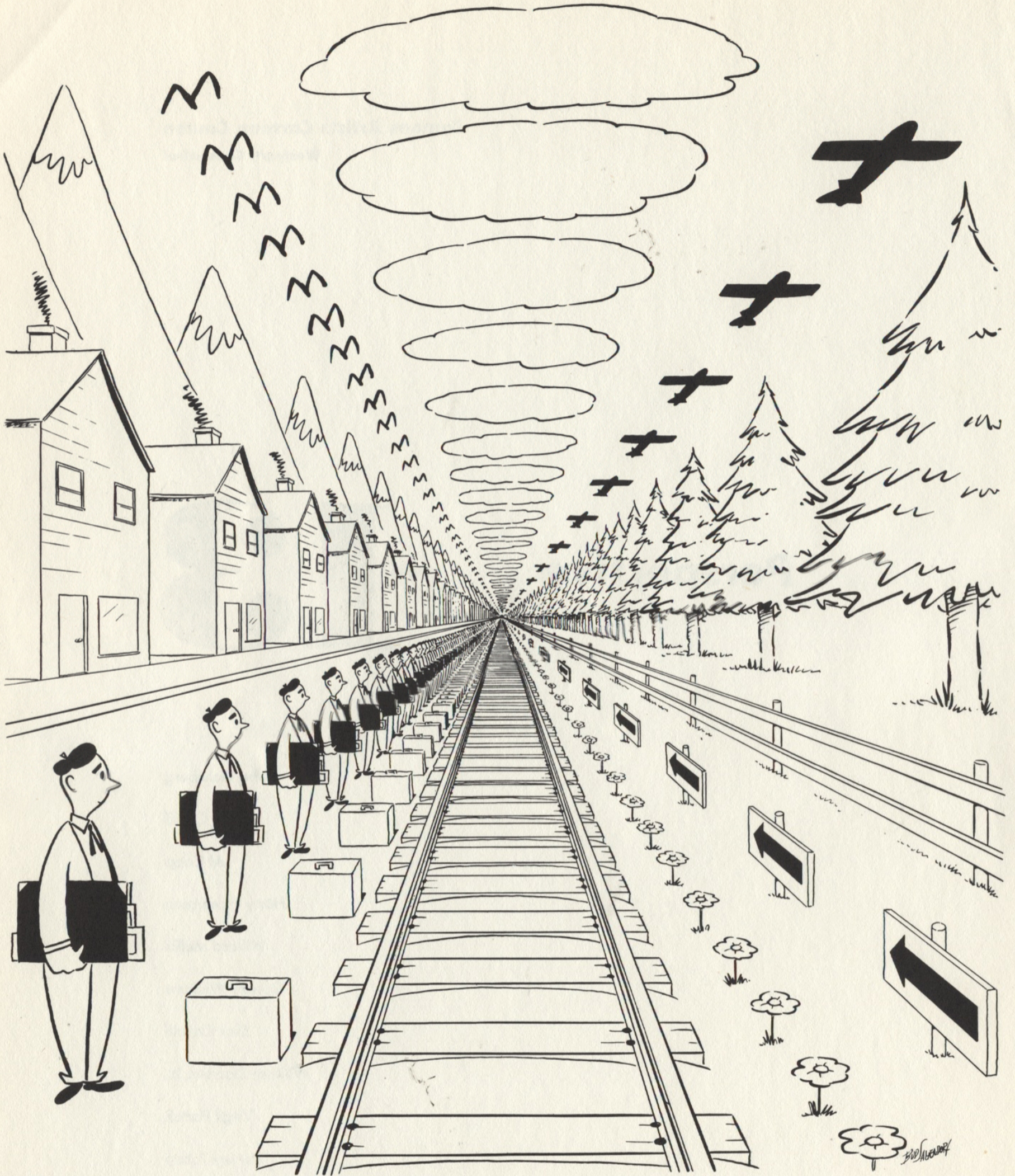
Everything appears smaller as it gets further away and parallel lines meet at a point on the horizon. This is called the vanishing point
